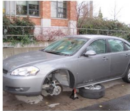
Figure 3. To test ECU behavior in a controlled environment, we immobilized the car on jack stands while mounting an attack.
